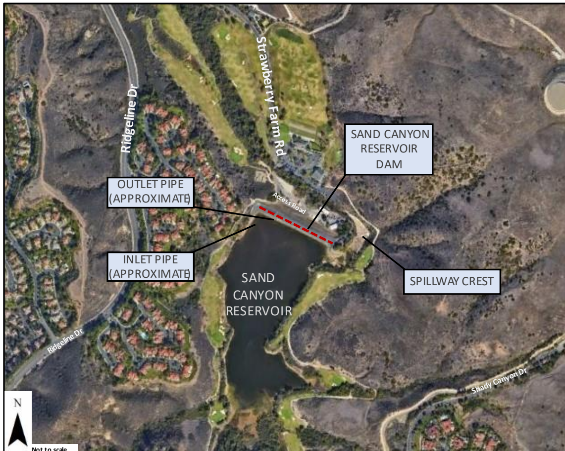
Figure 4-1 Schematic of Sand Canyon Dam
