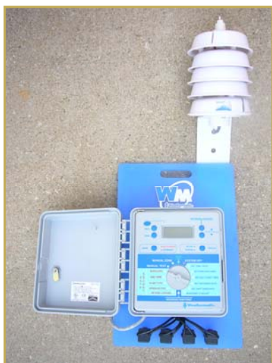
Weather-Based-Irrigation-Controller or smart controller for landscape irrigation.
