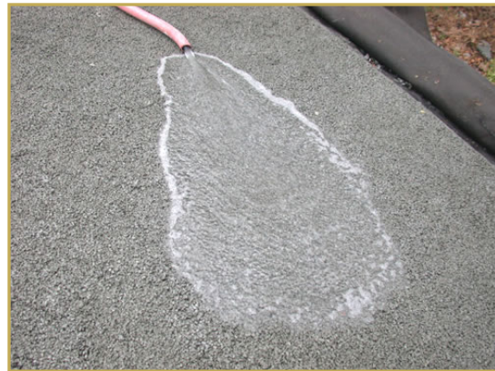
This is an example of porous concrete. Water percolates through the concrete and into the soil instead of running off into the stormdrain system. Courtesy of The Southeast Cement Association
