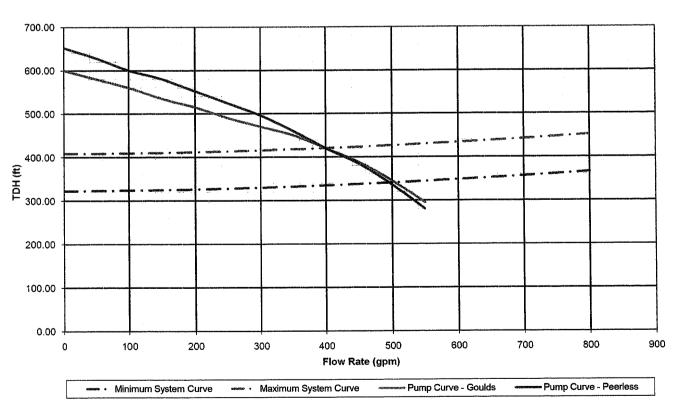
Pump/System Head Curves Goulds, 8RJLC, 5 Stage, 3500 rpm, 60 hp, 4.98" Impeller Peerless, 7HXB, 8 Stage, 3500 rpm, 60 hp, 4.43" impeller
