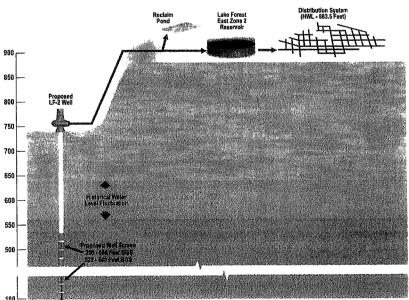
Kennedy/Jenks will design the well pump/motor to provide optimized production over range of water level conditions.
