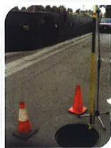
A Probe is Used to Measure the FOG Accumulation in a Grease Interceptor
