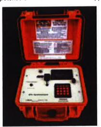
four (4) galvanic CP segments as outlined in the RFP's Project Description. The survey will measure on and instant off potentials by interrupting the cathodic protection current using GPS synchronizable interrupts. The interrupt cycle will have a minimum 80% duty cycle to minimize depolarization of the pipe during the survey.
