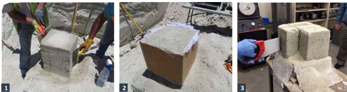
1-2. At Trampas Canyon Dam – Recycled Water Reservoir, AECOM gathered a carving block sample of bedrock for lab testing. 3. Preparing specimens in lab for engineering property testing.
