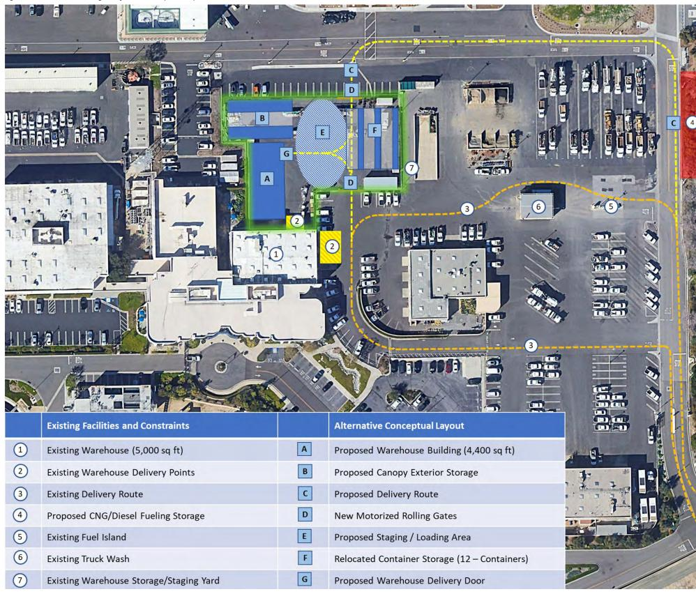
Figure 2 - Conceptual Layout and Project Site Constraints
