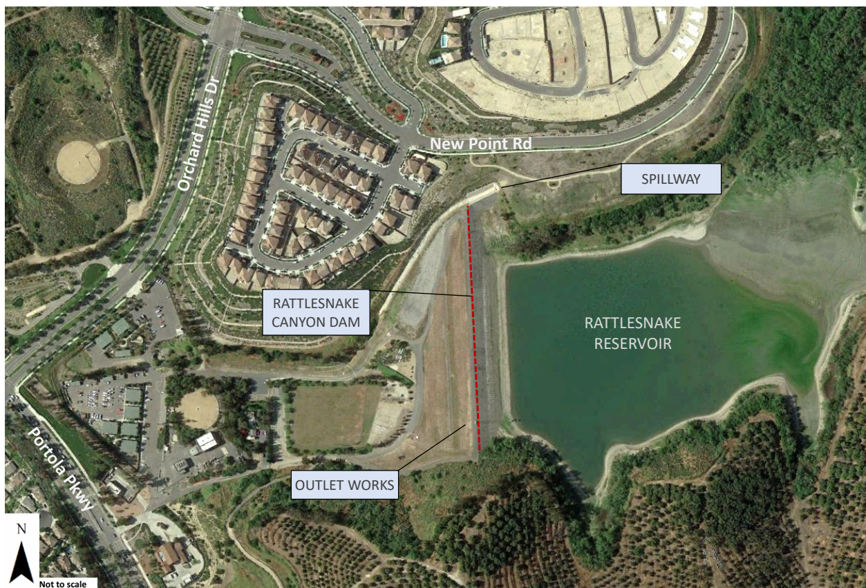
Figure 4-1 Schematic of Rattlesnake Canyon Dam
