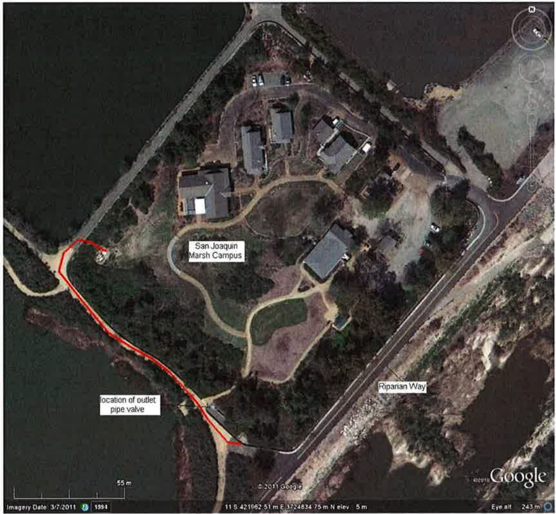
Figure 1: Proposed alignment of new electrical conduit (red line) for the San Joaquin Marsh Outlet Pipe Valve Replacement Project.
