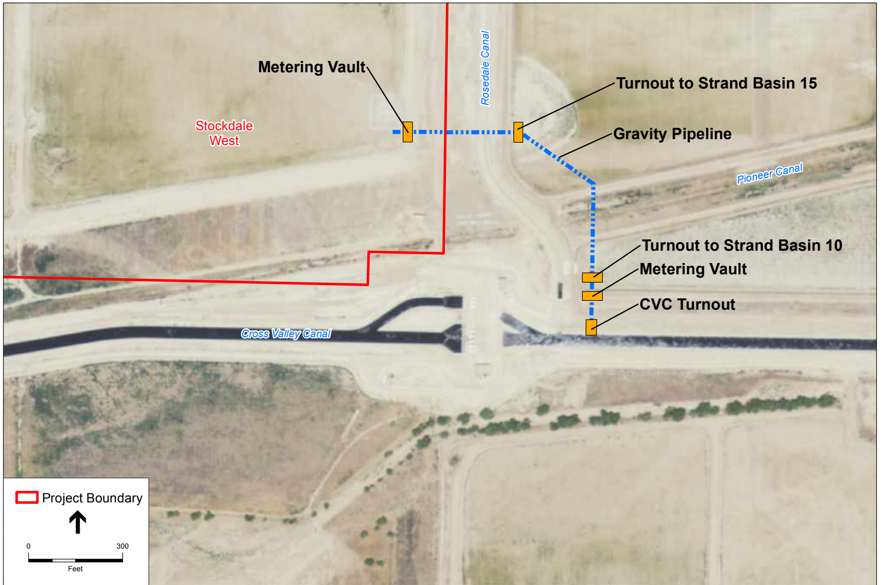
Figure 2-5 Proposed Stockdale West Gravity Turnout
